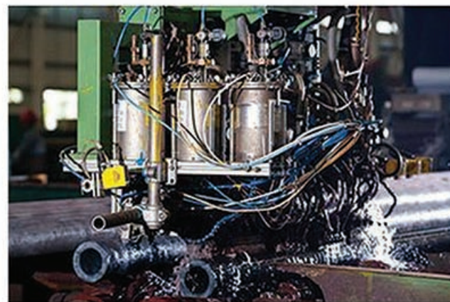
钻杆超声波检测 Ultrasonic test for Drill pipe
