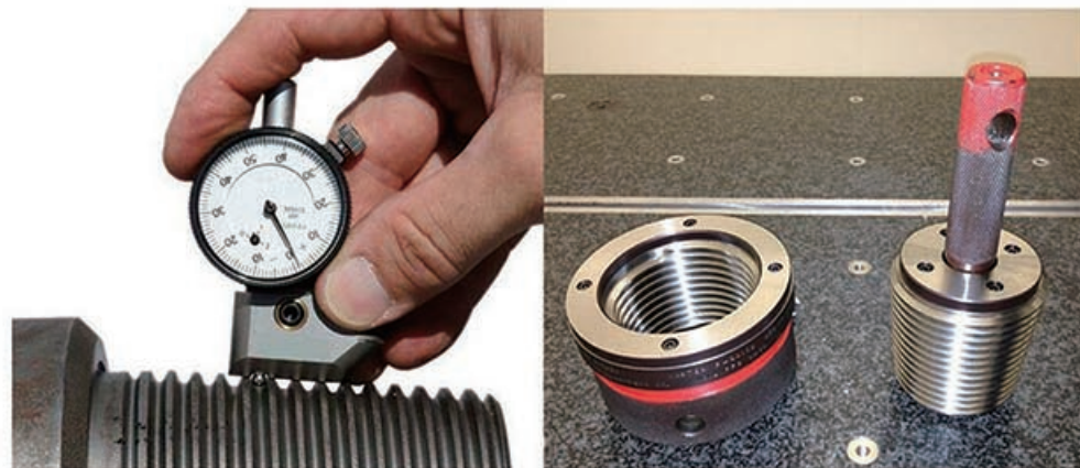
螺纹精度检测 Thread standoff inspection
